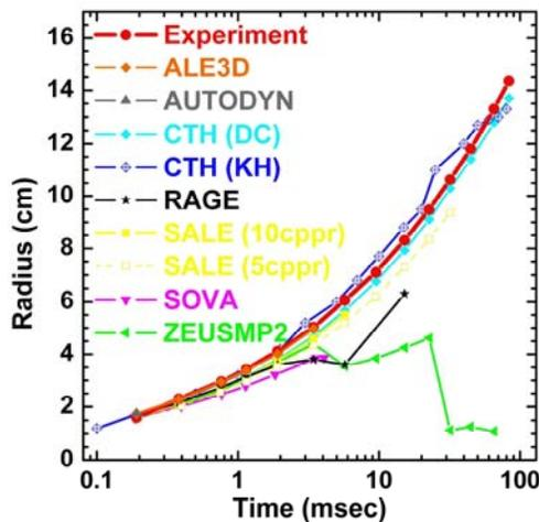
**Fig. 1:** Crater radius versus time for a 4.64 km/s impact of a glass sphere into water.
