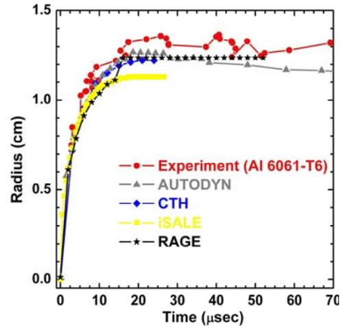
**Fig. 2:** Crater radius over time for a 7 km/s impact of an Al sphere into Al 6061-T6.
