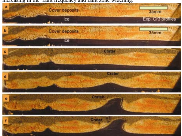
Fig4- The profiles of the Model by author in Fig3 show that any fracture on Mars may result to ice-salt mixture rising. The ice evolve from a pillow(c,d) to a narrow conical asymmetric diapir(e,f).The extension rate was high in this experiment. With increasing extension% the size of rising ice increased both in the crater and in the extensional faults in the left hand side. The top of the model (consist crater) covered by grey sand for better understanding of internal and external structures after impact.
