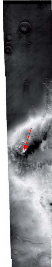
Figure 4: Result of spectral angle mapper. Brighter grey indicates a higher similarity to the reference spectrum taken at the red arrow.
