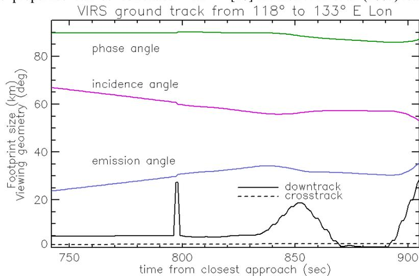
Figure 1. This plot is a description of the MASCs observations over the region to be imaged by MDIS during the color photometry sequence. The Visible and InfraRed Spectrograph (VIRS) component of MASCs, which covers the spectral range 320-1450 nm at 5-nm spectral resolution, will observe this region over a phase angle range of 85° to 90°, with the incidence and emission angle values ranging as shown. This data set overlaps the MDIS observations in both spectral and phase angle regimes.
