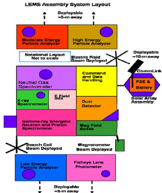
Figure 1: Schematic of one of Lunar Environmental Monitoring Station (LEMS).
