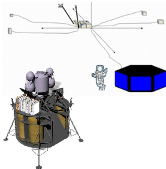
Figure 2: Schematic of deployed Lunar Environmental Monitoring Station (LEMS).
