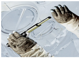
Figure 1: SPARCLE tool being used by astronaut to clean a glove in the airlock.
