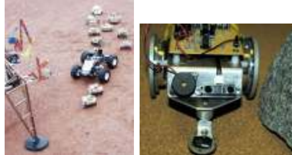
Fig. 6. Swarm of various Husar rovers work around the Hunveyor (a). This Husar-2 rover has a GP2D12 sensor to measure distance from rocks. All these are student works [6].
