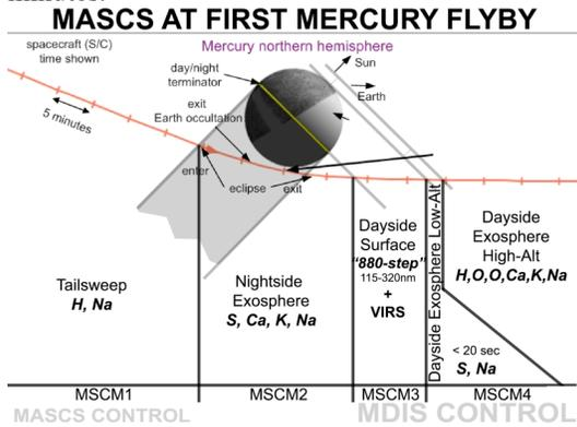
Fig 1. The orange line shows MESSENGER's trajectory near closest approach during the first Mercury flyby. Ticks mark 5-minute intervals. Vertical lines delineate boundaries of the four MASCS observing sequences. Sunlit surface observations are performed during MSCM3.
