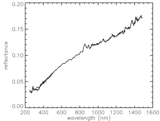
Fig 3. MASCS observation of lunar reflectance obtained during Earth flyby. The field of view of the instrument was centered at latitude =  $-10^\circ$ , longitude =  $-110^\circ$ , which is located on the far side as viewed from Earth, and the phase angle was  $65^\circ$ .
