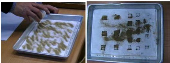
Fig. 1. After dispersing the mixture on the magnetic carpet (here white sheet) the magnetic component of the dust was adhered above the magnetic squares.
