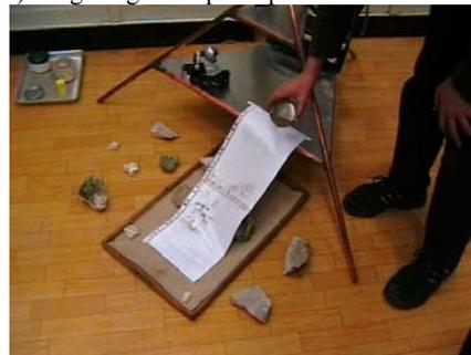
Fig. 2. Experiment arrangement with early version of Hunveyor-9. This position of the carpet is in a gentle slope. The magnetic carpet here is a white sheet with patterned magnet squares fixed inside the carpet.
