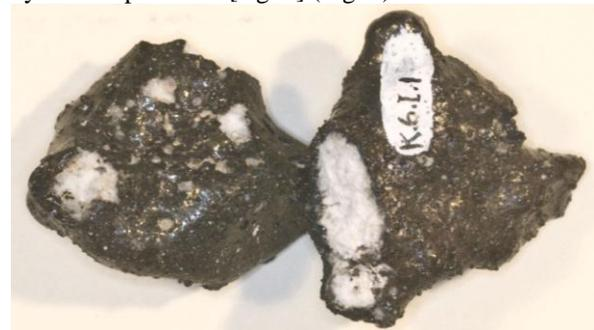
**Fig. 2.** Samples of impact melt coating matrix from the Wabar impact crater in Saudi Arabia. Image 6 cm width.
