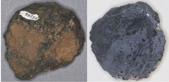
**Fig. 3.** Impact melt clast (6 cm diameter) surface (left image) and cross section (right image) from Henbury, Australia. Note the layered texture.
