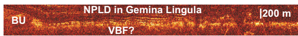
Figure 2. Portion of a SHARAD radargram over Gemina Lingula from orbit 5297, traversing Planum Boreum from \sim 85^\circ\text{N} , 45^\circ\text{E} (left) to \sim 79^\circ\text{N} , 21^\circ\text{E} (right) and showing the basal contact zone. Abscissa is distance along ground track, while the standard time (range) delay of the ordinate has been converted to depth, assuming the subsurface propagation medium has a real dielectric constant of 3.
