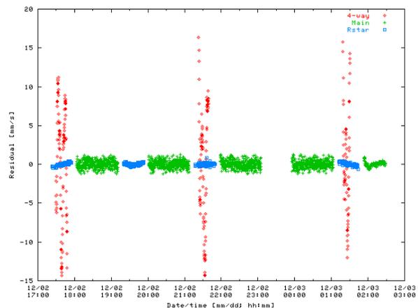
Figure 2. Doppler residuals for December 2-3 arc. Blue: Rstar 2-way, Green: Main satellite 2-way, Red: Main satellite 4-way. The 2-way Doppler data of the Main satellite are from the GN station except for the last pass starting at 02:00 December 3.
