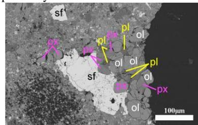
Fig 2. BSE image of an olivine-rich aggregate in the matrix. The aggregate consists of olivine, pyroxene (px), plagioclase (pl) and large sulfide (sf), typically with 120° triple junctions.
