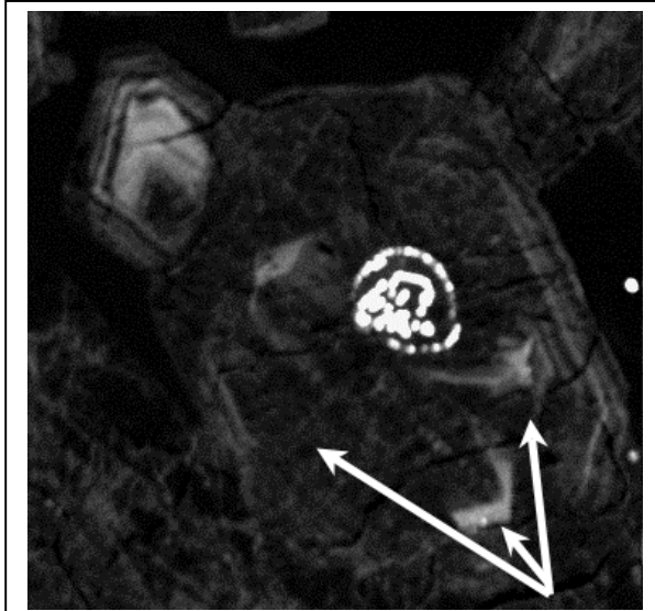
Fig. 2. P K_{\alpha} X-ray map of glomerocryst in RBT 04262. Bright rosettes are part of a melt inclusion; arrows point to possible ghost crystals. FoV: 370x380 \mu m.
