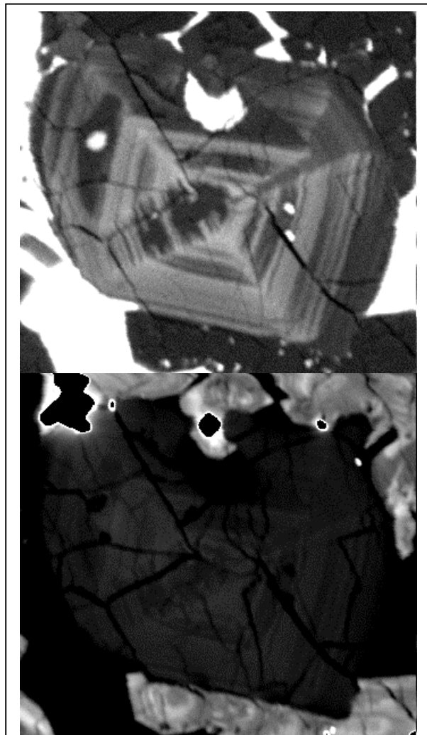
Fig. 1. P (top) and Cr (bottom) K_{\alpha} X-ray maps of olivine-phyric shergottite Y980459. Bright white areas inside the grain in the P map are melt inclusions. Field of view (FoV): 350x310 \mu\text{m} .
