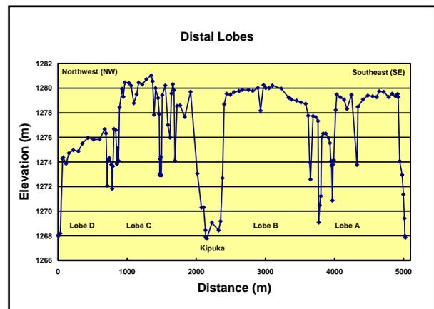
**Figure 2.** Topographic cross-section across four of the distal lobes from DGPS data.
