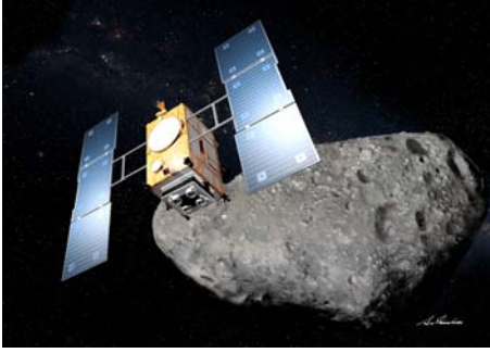
Fig.2 Artistic image of Hayabusa-2. The appearance of the spacecraft is almost same as Hayabusa, but a flat high gain antenna is used.
