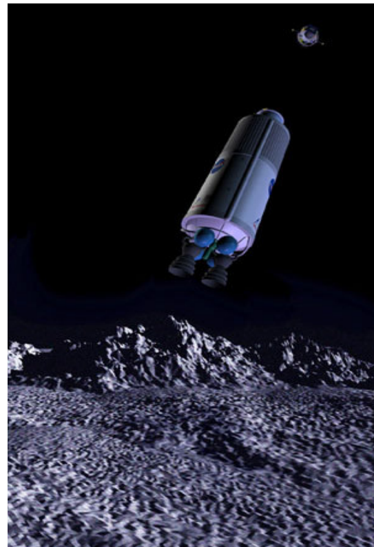
Figure 1. Artist concept of the EDUS (a Centaur upper stage) on its final descent toward the moon. The smaller Shepherd-ing Spacecraft (S-S/C) is shown in the upper right hand corner of the image. The S-S/C will characterize the morphology, dynamics and composition of the ejecta plume using nine instruments, including five cameras (1 visible, 2 NIR, 2 thermal), three spectrometers (1 UV/Visible, 2 NIR) and a flash radiometer.
