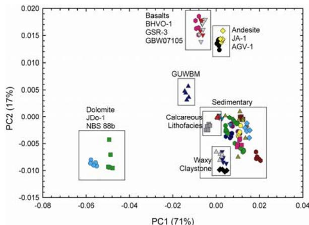
**Figure 2:** Principal Components Analysis (PCA) for all of the samples and standards explored in the paper. PCA can be used to develop a predictive model for rock types. PC1 and PC2 are dominated by variations in Ca, Mg, Na and Ca, Mg, Fe, respectively
