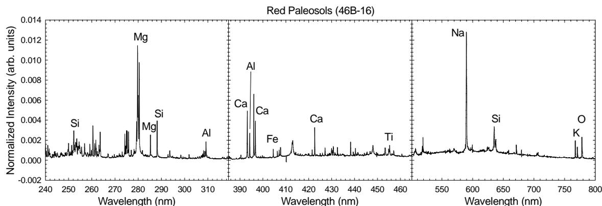
**Figure 1:** Representative LIBS spectra (from three different spectrometers) from a red paleosol (46B-16) at a 9m standoff distance. Most LIBS spectra are similarly spectrally rich and many of the major element emission lines are identified.
