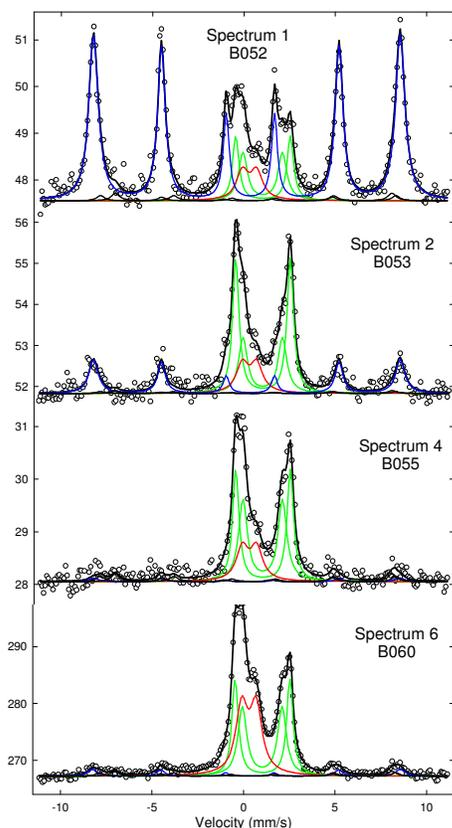
Figure 1. Counts data (o) with full function and site model subpectra (lines) for representative simfit spectra of the set B052–B056, B060. Hm (blue) is strong in spectrum 1–2; Ol, Px (green) in 2–4; npOx (red) in 6; and two weak sextets most clearly seen in 1 comprise the (Mt1, Mt2) contribution. The ordinate is kilocounts.
