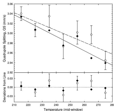
Figure 2. Variation of fitted quadrupole splitting for olivine in sample A050. Shown (top) are QS from six single-spectrum fits (open circles with error bars) and from simfits to the same data set (filled diamonds). The fitted linear fit trend lines are also shown. Deviations from the trend lines (bottom) demonstrate improved precision for the simfit values.
