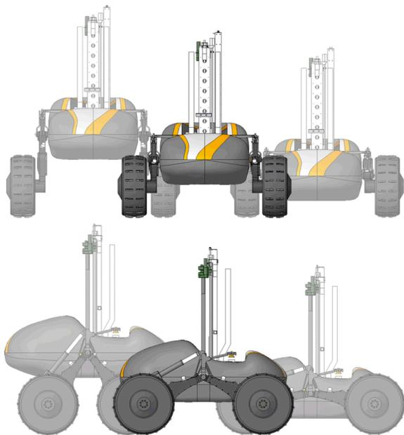
Figure 3: Schematic of Scarab in its range of suspension heights
