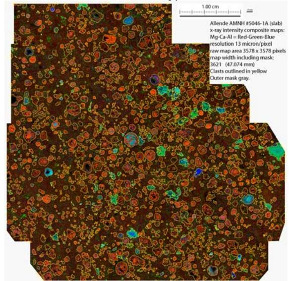
**Fig. 1:** Mg-Ca-Al composite x-ray mapping of slab 5046-1A, with clasts outlined in yellow.
