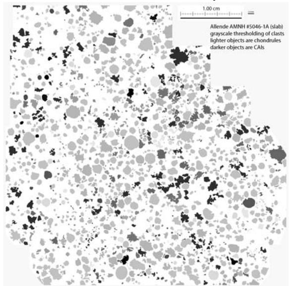
**Fig. 2:** Grayscale-coded clast output that is input into pixel-counting software.
