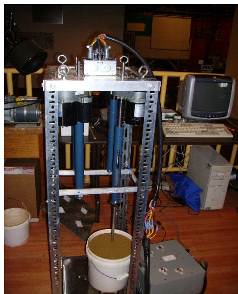
Figure 2. Constant velocity penetration test apparatus.
