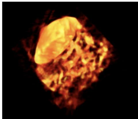
*Figure 1. Stardust Track 12 (C2044,0,52). Two-dimensional image from the 3-D tomographic reconstruction using X rays above the Fe K-absorption edge. Particle direction of travel is from lower right to upper left. Agglomerated material is visible in the wake of the prolate spherical particle.*
