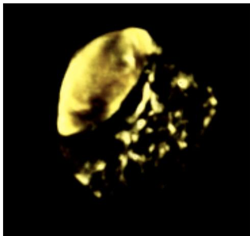
Figure 2. Two-dimensional image of the Track 12 terminal particle using x-rays of 7100 eV, below the Fe K-absorption edge. The ~100 nm particles do not absorb as strongly at this photon energy.
