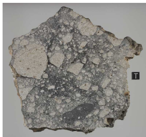
Figure 3: Complete 19 cm slice cut parallel to the top surface shown in Figure 2. Note metal grains with minor rusty staining in leucogabbroic clasts and matrix.
