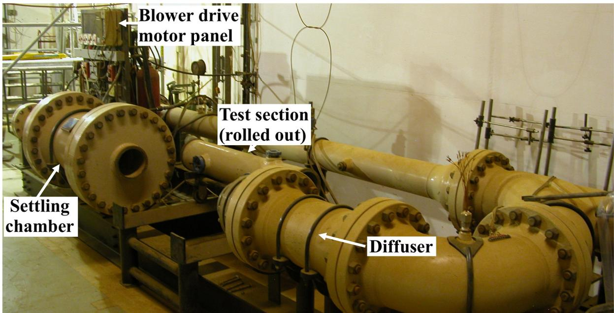
**Figure 1:** Photograph of the Venus Wind Tunnel (VWT) at the NASA Ames Research Center Planetary Aeolian Laboratory (PAL). The fan is just off the image to the middle right. The gas supply lines are behind and to the right of the drive motor panel.
