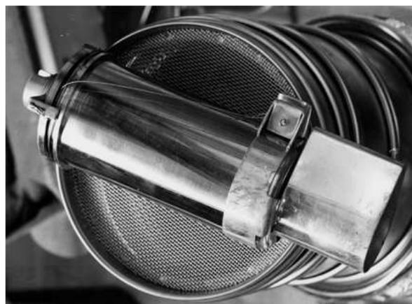
Figure 2. The SESC container (Special Environment Sample Container).
