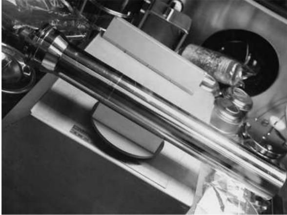
Figure 3. The CVSC (Core Vacuum Sample Container).
