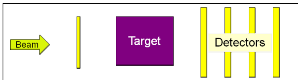
Figure 1. Schematic relationship of the high-energy beam, the sample as the target, and the particle detectors.
