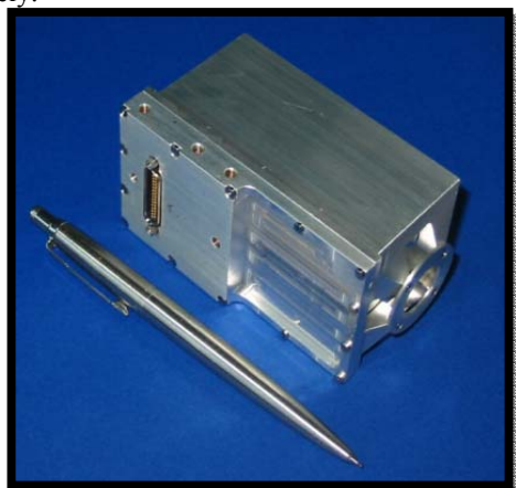
Figure 1: The MER type version of the MIMOS II sensorhead with approximate dimensions 95 mm x 45 mm x 40 mm.
