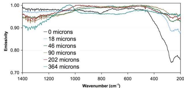
Figure 5. TIR spectra of oxidized surface with incremental dust loading. Strong absorption features are not completely masked until after 364 microns of dust are applied.
