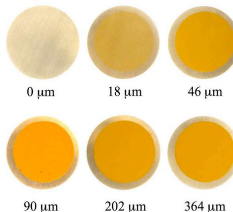
Figure 4. Dust thickness is measured using an aluminum disc adjacent to the specimen in the airfall chamber. The rate of opacity development in visible light is similar to that of the infrared.
