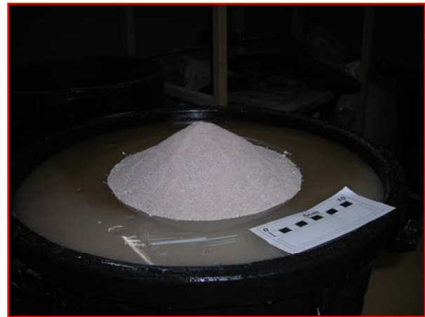
Fig. 1 Photograph of the simple experimental setup used to produce flank terraces. A conical load of quartzose sand was placed upon a deep layer of viscous silicone and allowed to flex. Cone geometry is approx. 16 cm in basal diameter, and 8 cm high.
