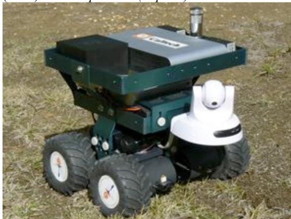
**Fig. 1.** 4WD remote controllable rover platform as a test bed for lunar and martian surface operations.
