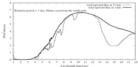
Fig. 3a. Disk-integrated spectra including the weighted contribution of the surface element orientation for Earth. The planet is seen from the south pole.
