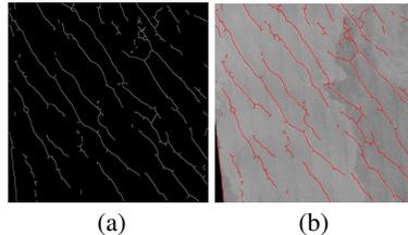
**Figure 4** - (a) Final result of automatic detection of wrinkle ridges; (b) superposition of the wrinkle ridges on the original image.
