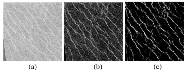
**Figure 2** - (a) Fractal dimension of the image on fig. 1; (b) threshold of (a) based on fractal value for wrinkle ridges ( $D \geq 2.68$ ); (c) area opening followed by reconstruction.
