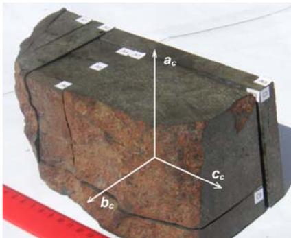
**Fig. 2.** Cutting plan of #15390,9 sample of Tsarev, where  $a_c$ ,  $b_c$  and  $c_c$  are coordinates of anisotropy.
