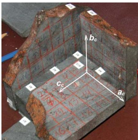
**Fig. 3.** Cutting plan of #15390,9 sample of Tsarev, where  $a_c$ ,  $b_c$  and  $c_c$  are coordinates of anisotropy.
