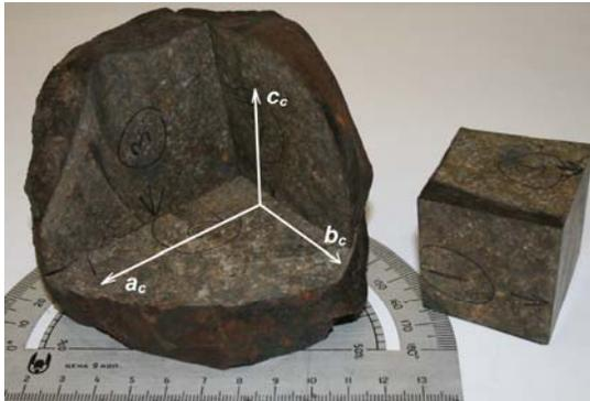
**Fig. 1.** Cutting plan of SAUH 001, where  $a_c$ ,  $b_c$  and  $c_c$  are coordinates of compressive strength anisotropy.
