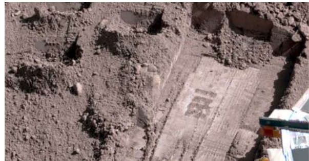
Fig. 1 – Surface Stereo Imager false color image of the Snow White Trench where back-hoe, scraping, and rasping succeeded for acquisition of the icy soil sample, Wicked Witch, for delivery to TEGA. The array of dark splotches at the bottom of the trench are ~1 cm wide rasp holes into icy soil. Rosy Red surface soils were acquired from the trenches visible on the upper left portion of the image.
