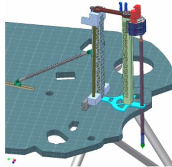
Figure 1: The heat flow probe. The system consists of a deployment stage, percussive head, telescopic rod with a sensor tube and an anchor/cone at the end.
