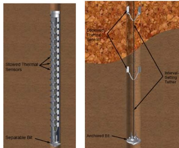
Thermal sensor anchors stowed within the penetrometer. Separable cone/bit deployed as a thermal sensor string anchor
