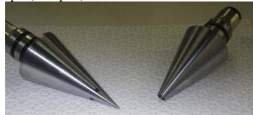
Figure 4: Cones with injector nozzles. Top left: 4 injector nozzles around the tip of the cone; Top right: central injector nozzle replacing the tip of the cone.
