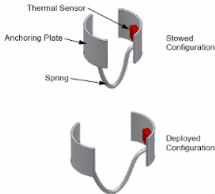
Figure 3: Individual thermal sensor emplacement anchors shown in stowed (top) and deployed (bottom).
