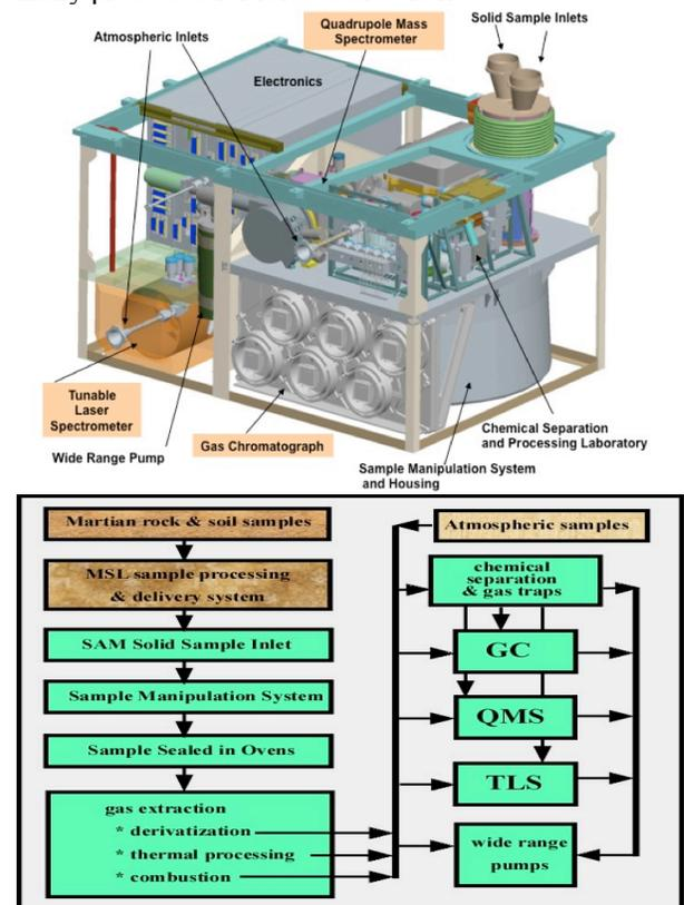
**Figure 1.** The layout of SAM's instruments and major supporting subsystems is illustrated in the top portion of this figure and the flow of gas and sample to the instruments illustrated in the lower panel.
