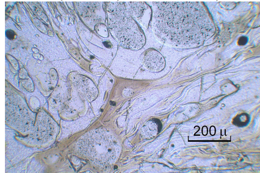
Fig. 2. Dynamic interfingering between types II (colorless) and III (brownish strips in the center) glasses. Popigai suevite, LH sample #1308, micro photo.
