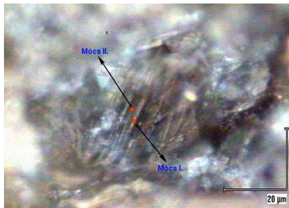
Fig. 1 Reflected light micrograph of PDF's in olivine from Mócs meteorite sample. (Two red solid circles correspond to the Raman analyzing points).
