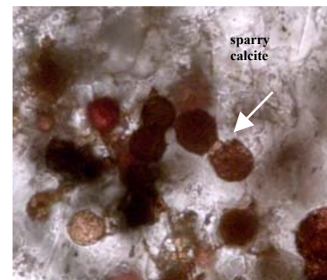
Fig. 2: Optical microscope image showing framboids. They are isolated or but some appear to be joined by a meniscus (arrow). Framboids range in size from 1-2 to 11 \mu m in diameter.
