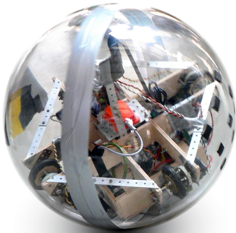
Fig. 1. The Hungarosphere rover is a transparent sphere with inner driving by 4 motors. It can follow any directions in any time.
