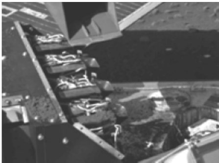
Fig. 2: Phoenix image from the Surface Stereo Imager showing delivery of soil from the robotic arm to the WCL cell.
