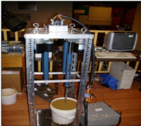
Figure 2. OPRA penetration test apparatus.
