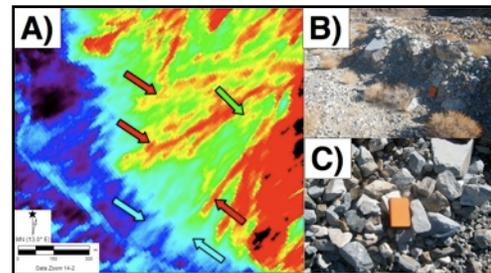
**Figure 3:** a)  $\Delta T$  map ( $\sim 2$  m/pixel) of Dolomite alluvial fan. Red arrows marks location of debris flow lobes. Green arrow marks location of remnant debris flow levees. Light blue arrows marks location of clast-poor debris flows. b) Debris flow levee near green arrow c) Grain size distribution of debris flow lobe near red arrow.
