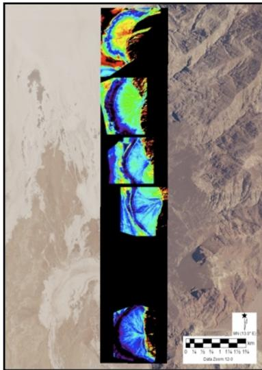
**Figure 1:**  $\Delta T$  map of alluvial fans on the east side of Death Valley near Badwater Basin. Warm colors indicate areas of high thermal inertia (inferred from lower  $\Delta T$  values), with larger grain size distributions while cooler colors indicate areas of low thermal inertia (inferred from higher  $\Delta T$  values) with smaller grain size distributions.
