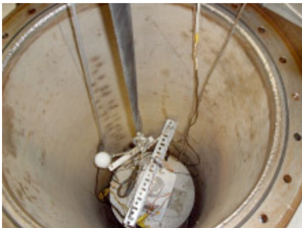
Figure 4. The Andromeda planetary simulation chamber will be used to test the probe in a space like environment, and perform in situ spectroscopic analysis of samples in the chamber
