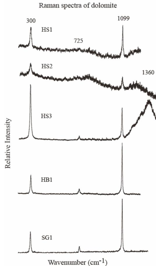
**Fig. 2.** Raman spectra of dolomite from 1) Haughton carbonate clasts within impact melt rock: HS1, HS2 and HS3, 2) Haughton carbonate bedrock from outside the crater HB1, and 3) Dolomite from St. Gotthard, SG1.
