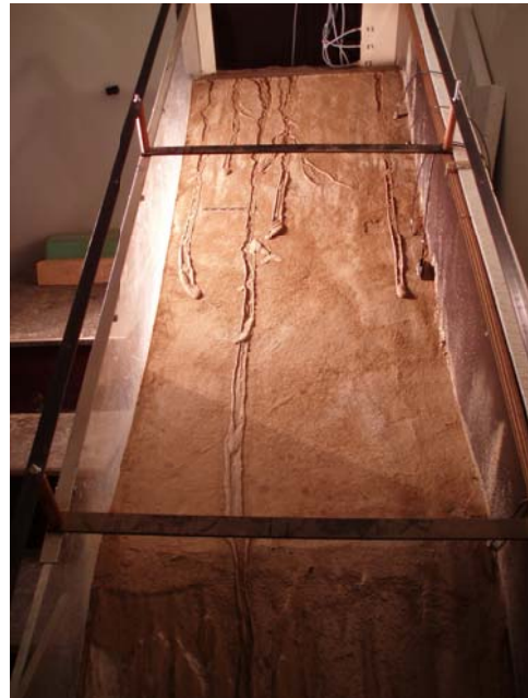
Figure 2. Close-up of the apparatus used in the physical modelling of debris flows.
