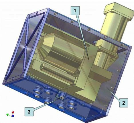
**Fig. 1.** Concept design of BTN/ISS detector unit [1- detector unit equal HEND/MO instrument; 2 – special frame for mechanical and thermal condition providing; 3 – montage holes for bracket]
