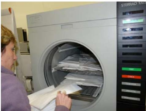
*Mars96 mission heritage (OPTIMISM Seismometer)*: for Planetary Protection aspects the seismometer team can benefit of Mars96 heritage in terms of procedures. Specific procedure has been validated using the Sterrad 100S® process (ASP Johnson and Johnson medical process). The procedure was used with reduced plasma phase. Sterilized equipments were packaged into two successive similar bags (qualified for the sterilization method).
