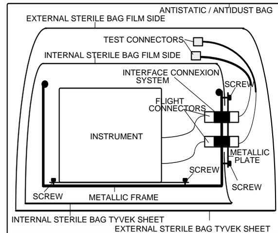
*Identification and description of controlled facilities* : Work of integration will be done in laminar flow hood within a clean room (ISO7 or better)
