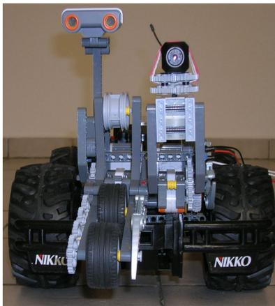
*Fig. 1. On the front of the rover there is an ultrasonic sensor of the obstacles before the rover. Upper arm). There is also the camera (right up) and there is the arm moving the indicator ribbon. The ribbon is rolled from one wheel to the other wheel while the arm is contacting the surface and soil. Camera observes the changes on the indicator ribbon colour.*
