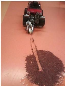
Husar-5 moves backward to prepare observation of the rolled indicator surface, which holds the information about the pH of the soil.
