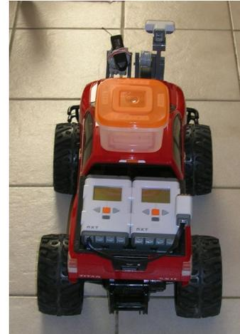
*On the back of the rover are the two „brains”, which control the movements and the motors of operation of the arms and they also receive the signals of the sensors. The water container is on the top of the rover.*
